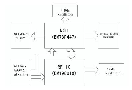
The encoder generates a digital code serially transmit (typical designation), The 12M crystal oscillator driver the base of MCU.MCU will read the status of Optical Sensor, Encoder and Buttons, then control the RF chip by thru the SPI Bus, and the Modulation type of RF chip is GFSK, the frequency of Modulation is 150 KHZ, and the output power of RF chip is -5dBm.
