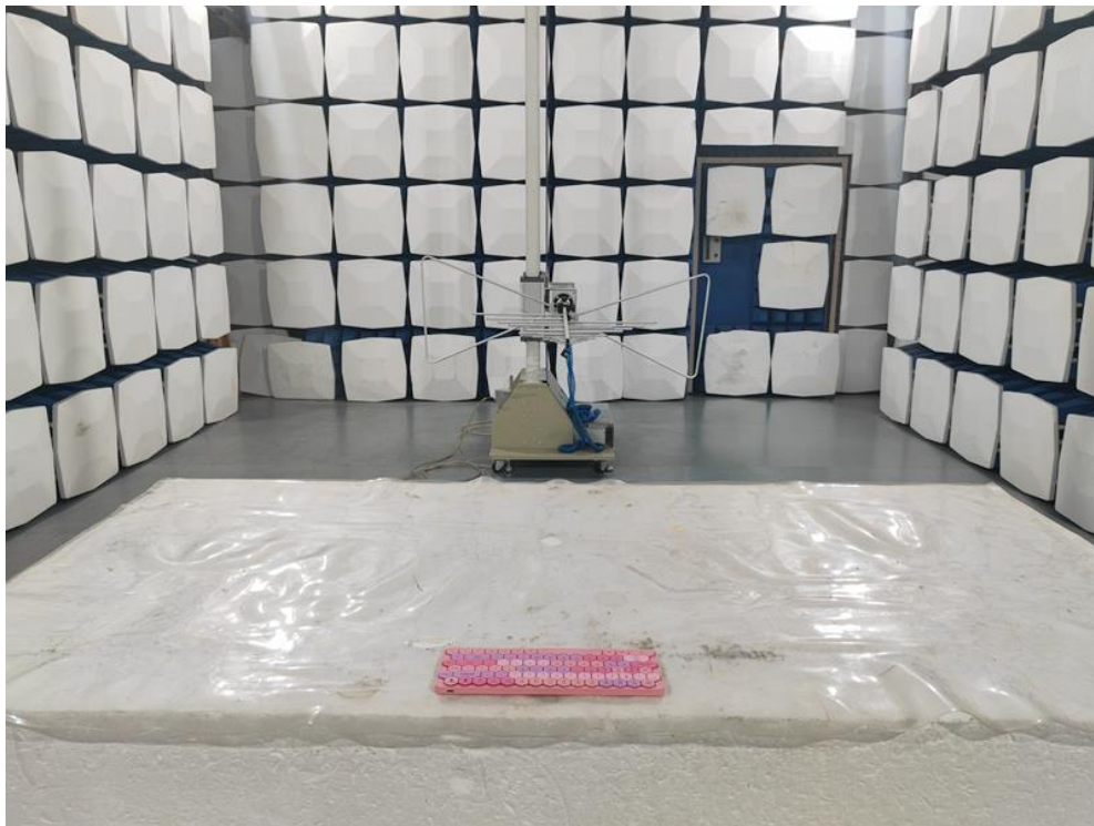
Radiated Emission Test Setup:
