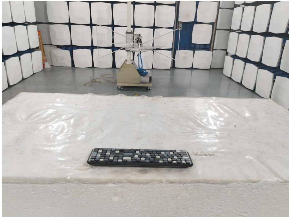
Radiated Emission Test Setup:
