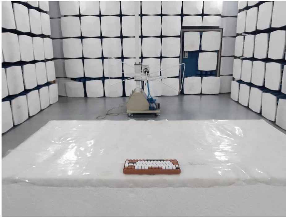
Radiated Emission Test Setup:
