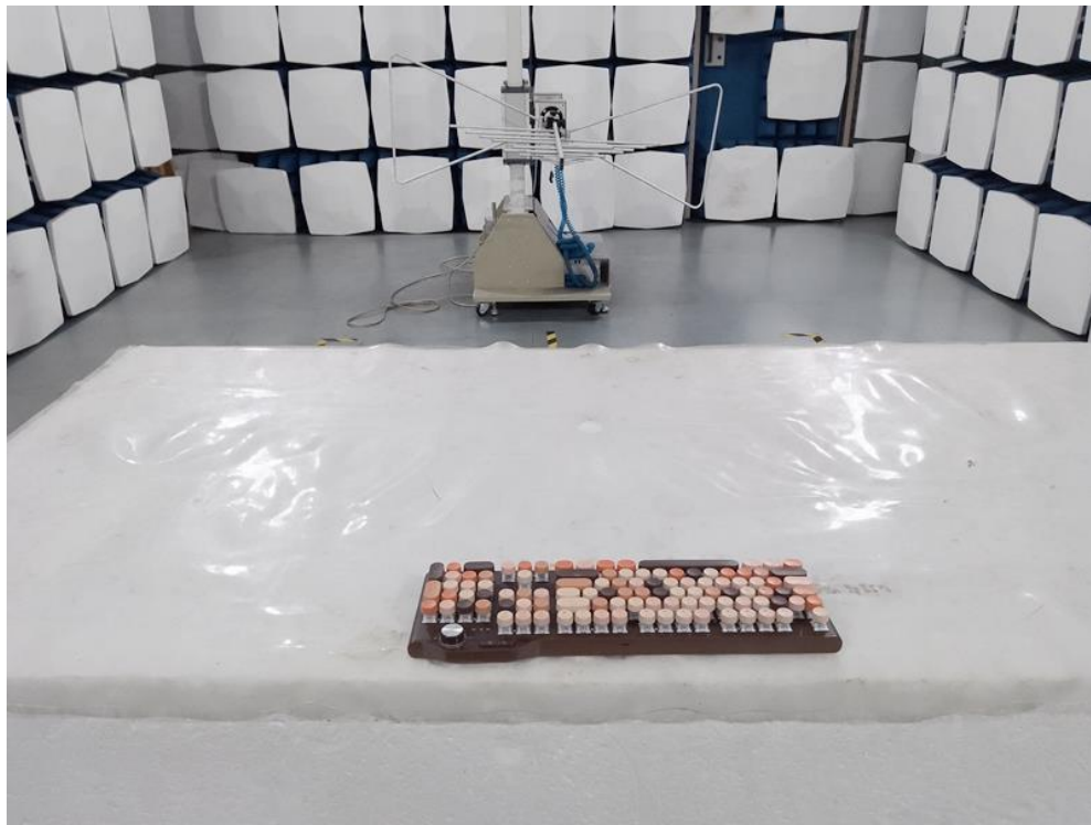
Radiated Emission Test Setup:
