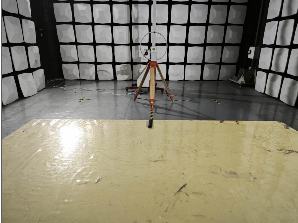
Test Photo Radiated emission (Below 30MHz)
