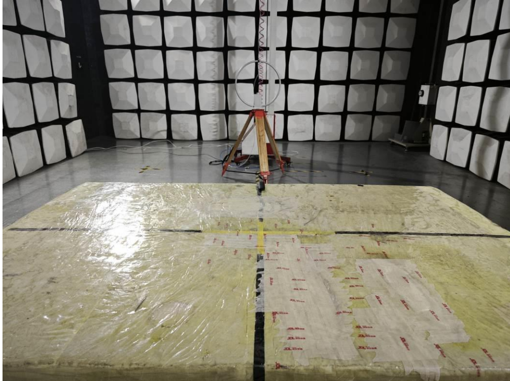
Test Photo Radiated emission (Below 30MHz)
