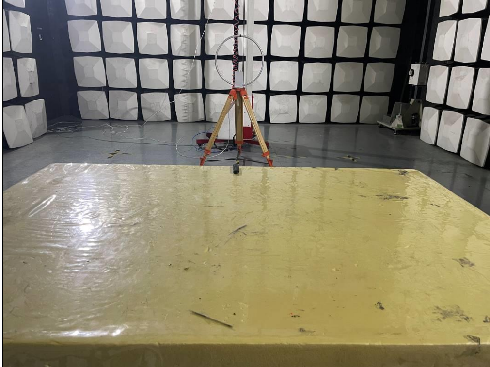
Test Photo Radiated emission (Below 30MHz)
