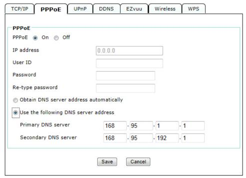
**IP** address: The IP address obtained at the PPPoE connecting with network.
