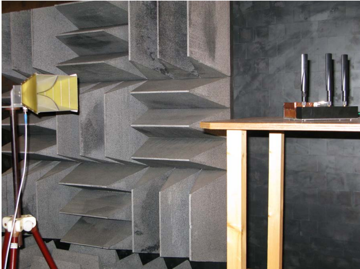
Photograph 3: Radiated emissions setup (>1 GHz)
