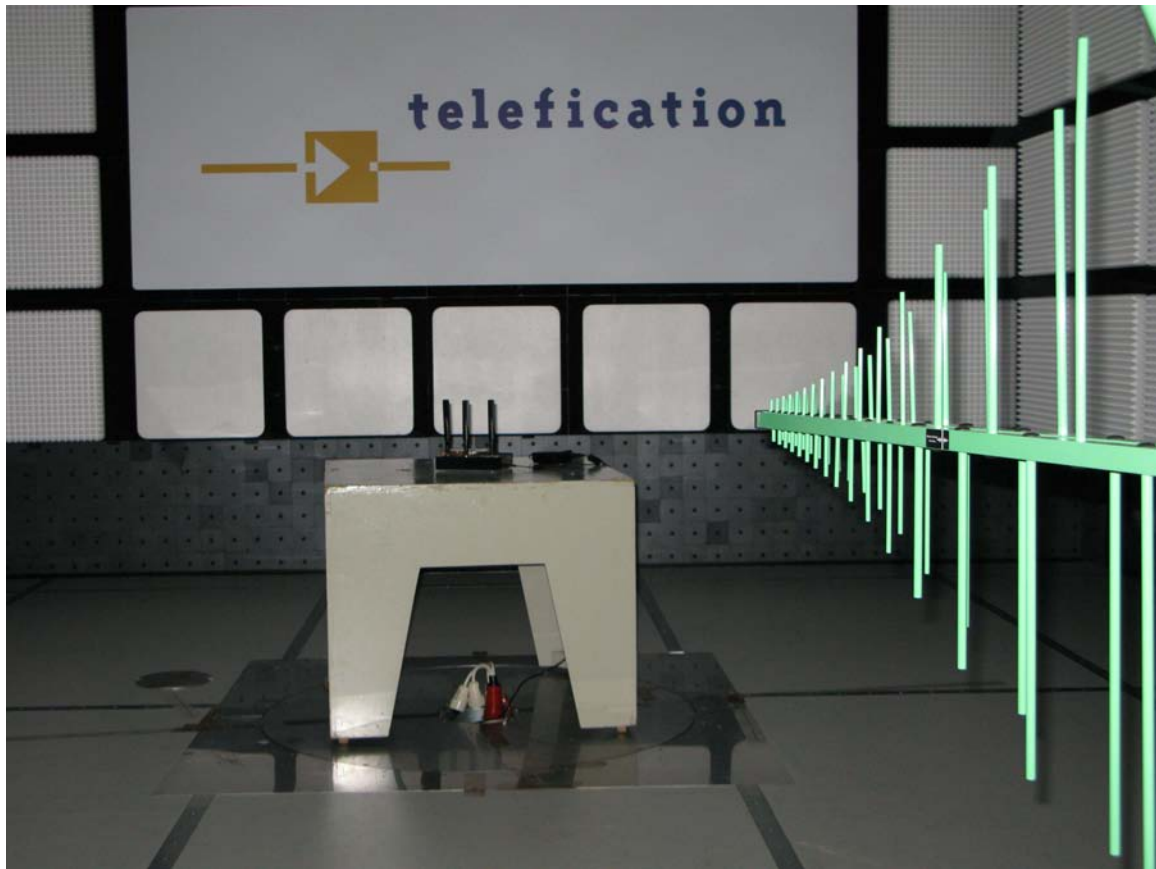
Photograph 2: Radiated emissions setup (<1 GHz)
