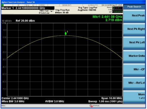
Modulation Standard:  $\pi/4$ -DQPSK (2Mbps) Channel: 78
