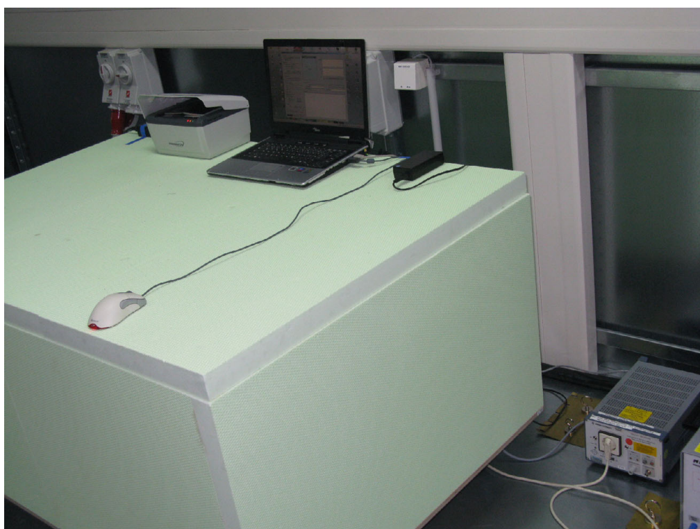
Figure 4 Arrangement for the measurement of conducted emissions
