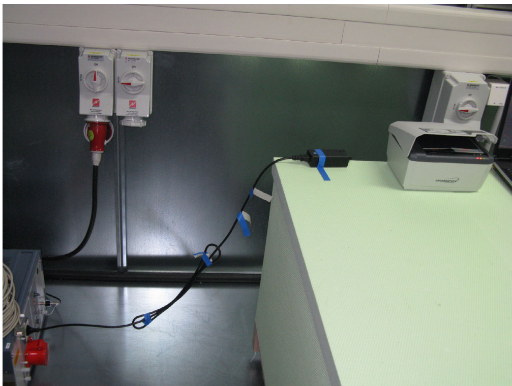
Figure 2 Arrangement for the measurement of conducted emissions
