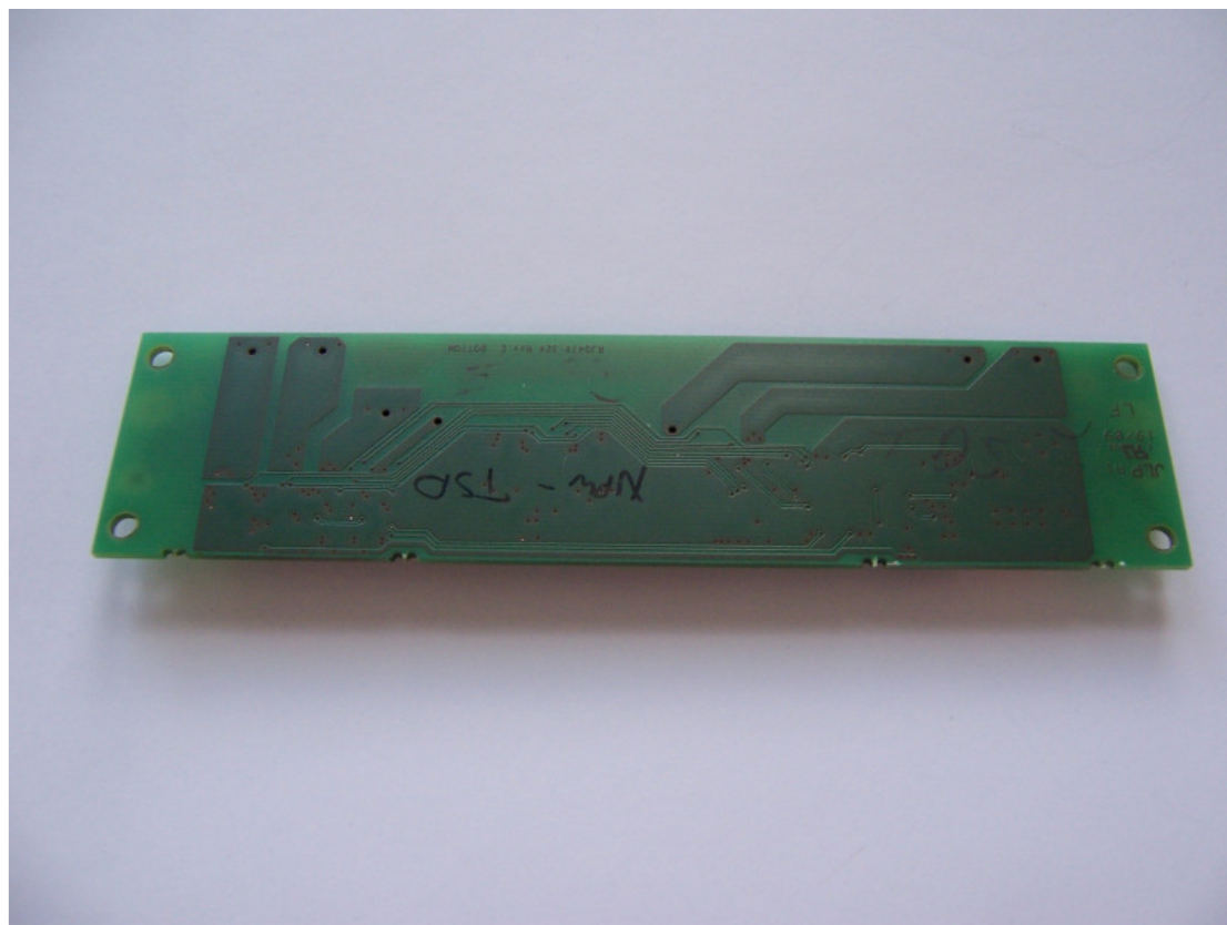
Figure 10 Illumination PCB, RJ0479:324.25 RevE, Rear
