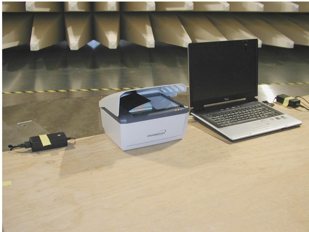
Figure 1 Arrangement for the measurement of radiated emissions
