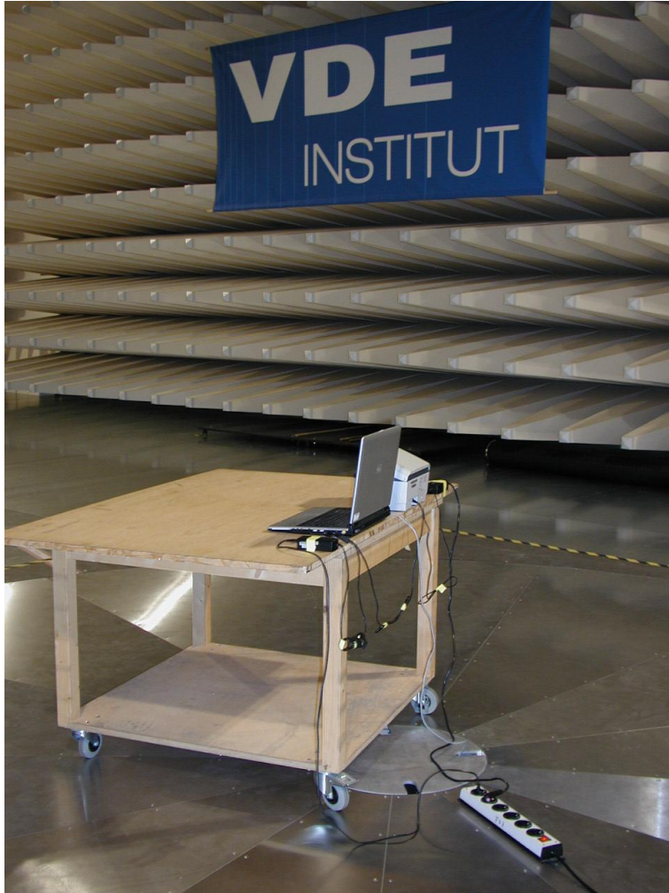
Figure 3 Arrangement for the measurement of radiated emissions
