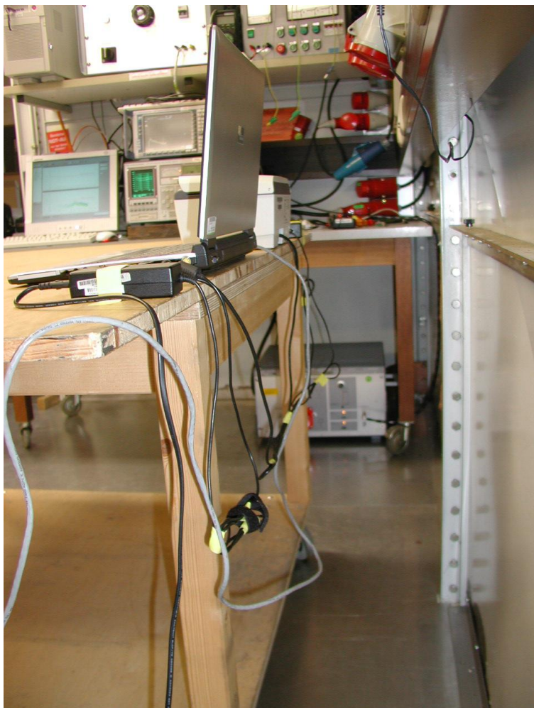
Figure 4 Arrangement for the measurement of conducted emissions
