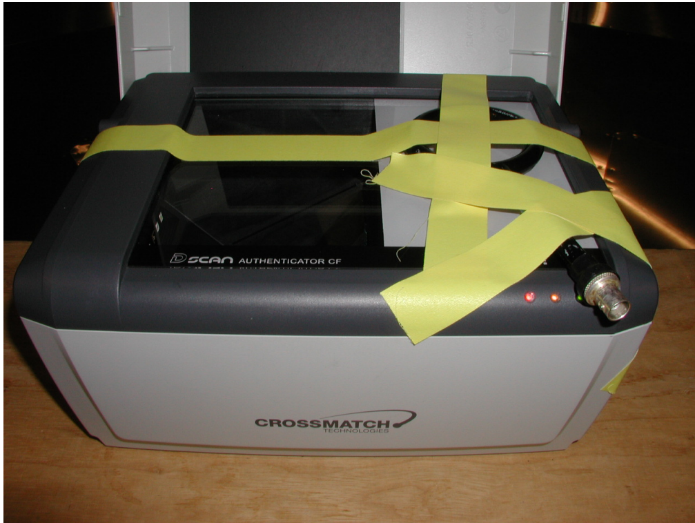
Figure 9: EUT with electrically shielded loop on the scanner surface for relative measurements in the environmental chamber
