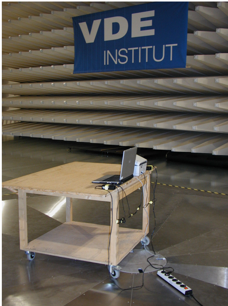
Figure 7 Arrangement for the measurement of radiated emissions
