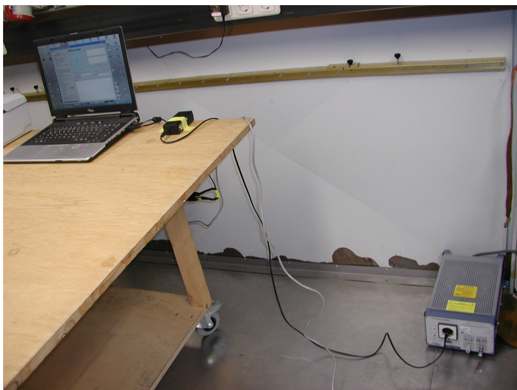
Figure 3 Arrangement for the measurement of conducted emissions
