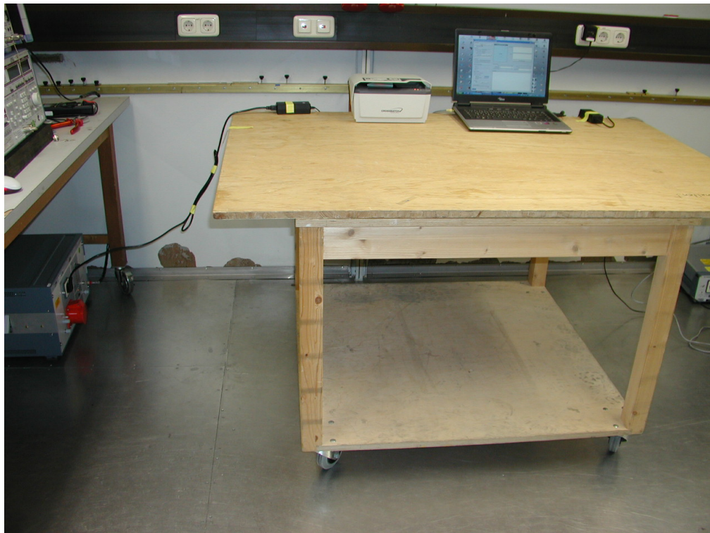
Figure 1 Arrangement for the measurement of conducted emissions
