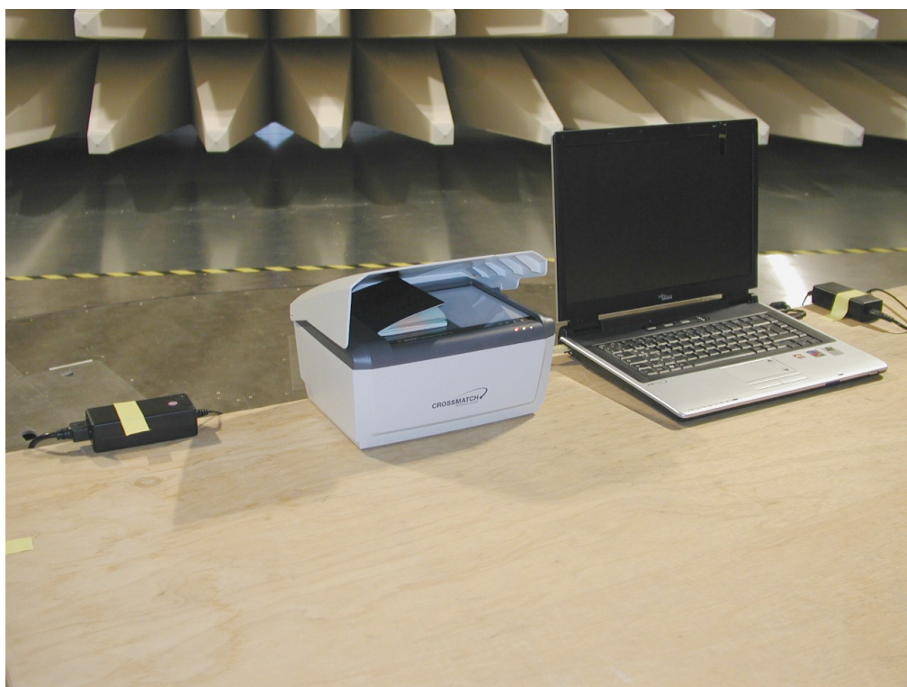
Figure 5 Arrangement for the measurement of radiated emissions
