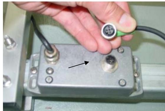
Remove the face plate of the KR2003; undo the screws and keep them in a safe place. Install the 1GB SD Card. Note: removing and replacing the SD card should be performed with the receiver unpowered.
