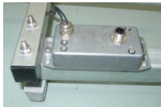
Connect 5 pole M12 connector – 3 poles signal; 2 poles power
