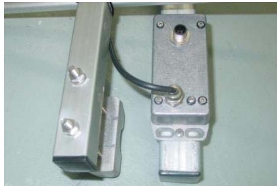
Place the box section with the electronics enclosure attached to it as illustrated below
