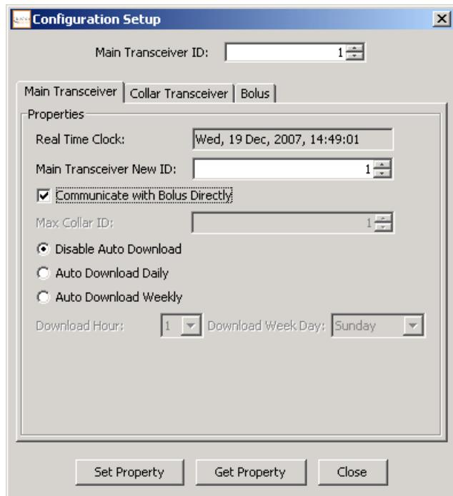
3. Make sure that the *Main Transceiver ID* corresponds directly to the transceiver being used. If not manually changed, the *Main Transceiver ID* will be set to 1 as a default.
