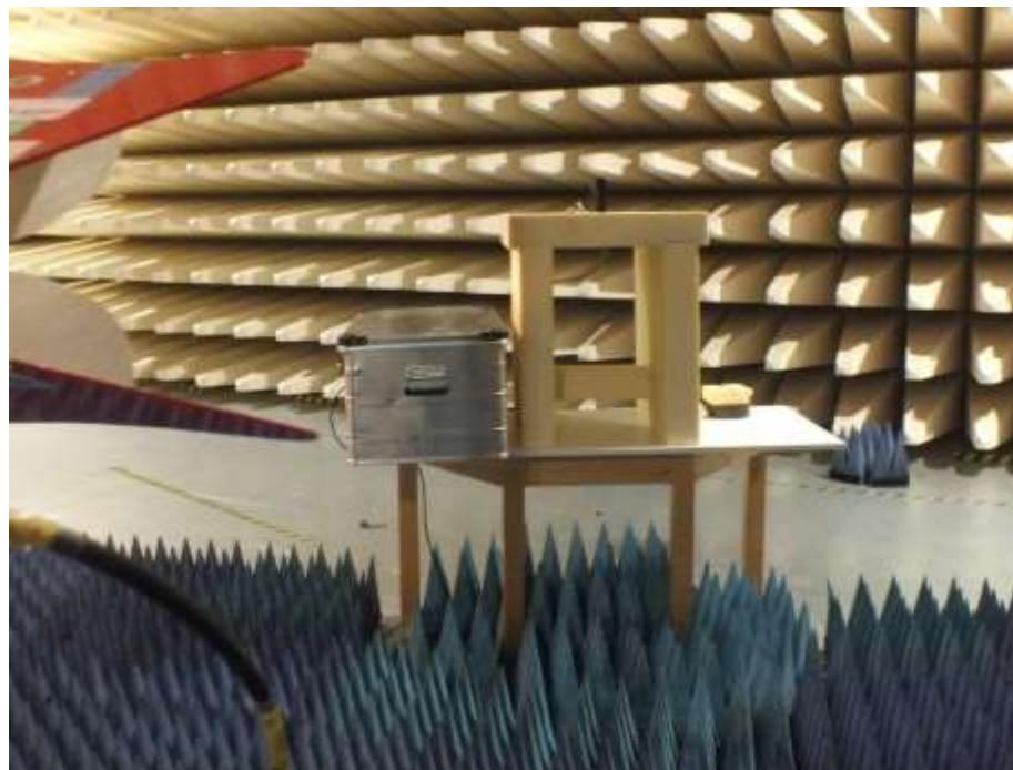
Test setup 18 GHz – 26 GHz
