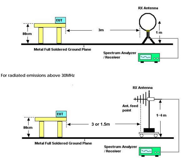
Above 10 GHz shall be extrapolated to the specified distance using an extrapolation factor of 20 dB/decade form 3m to 1.5m.
