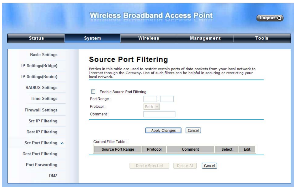
Figure 11 Source Port Filtering
