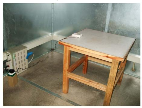
2.Radiated Emission Test Setup(Below 1GHz)
