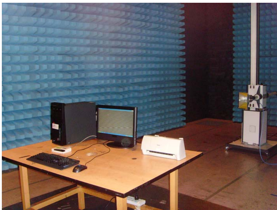
Radiated Emission Test Set-up (Above 1GHz)
