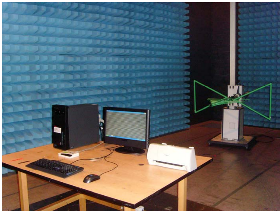
Radiated Emission Test Set-up (Below 1GHz)
