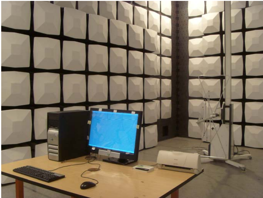
Radiated Emission Test Set-up (below 1GHz)
