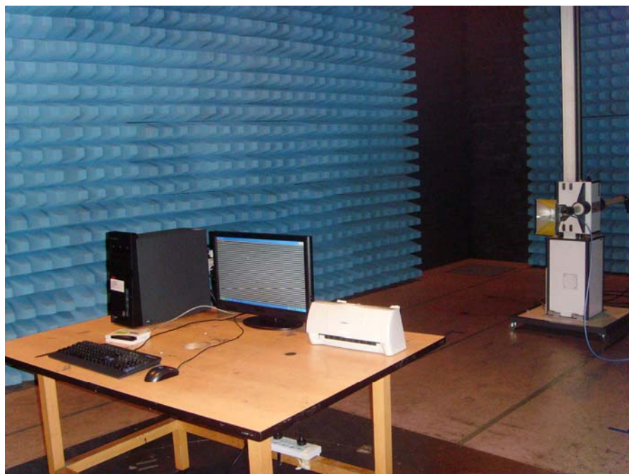
Radiated Emission Test Set-up (above 1 GHz)
