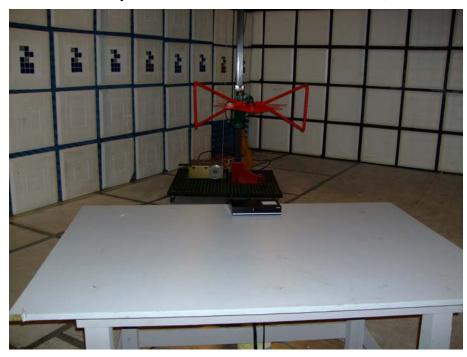
2. Radiated spurious emission measurement(Above 1GHz)
