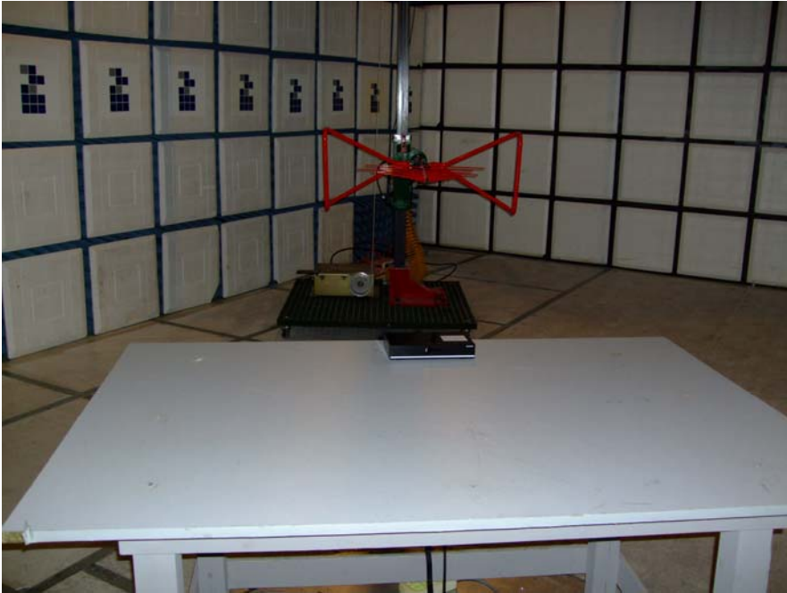
Radiated Emission Test Set-up(Below 1GHz)
