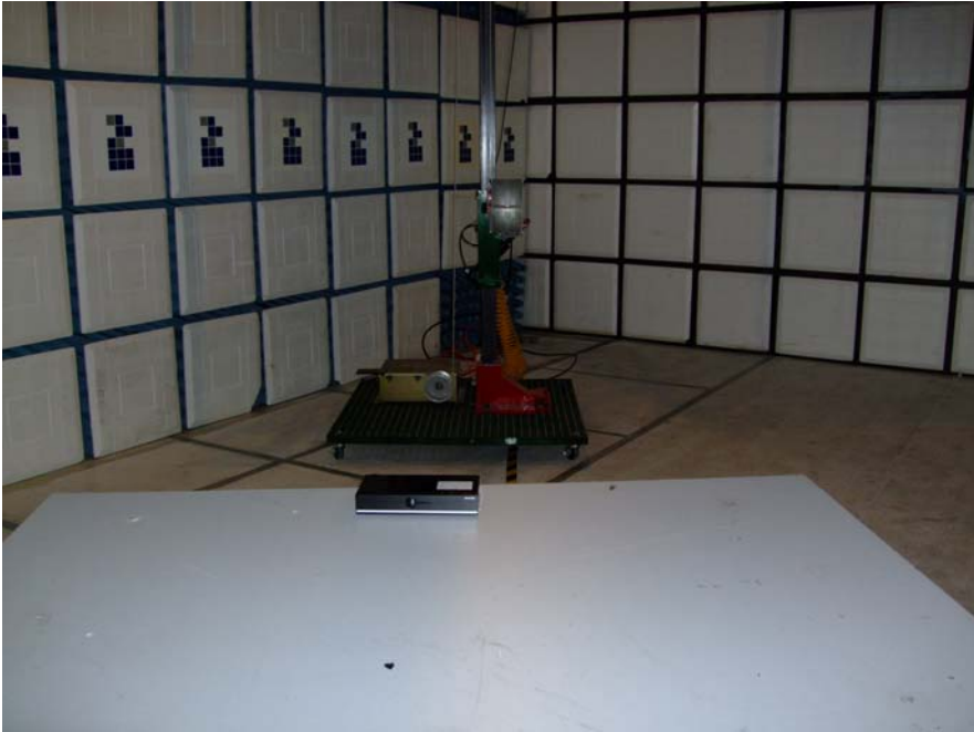
Radiated Emission Test Set-up(Above 1GHz)
