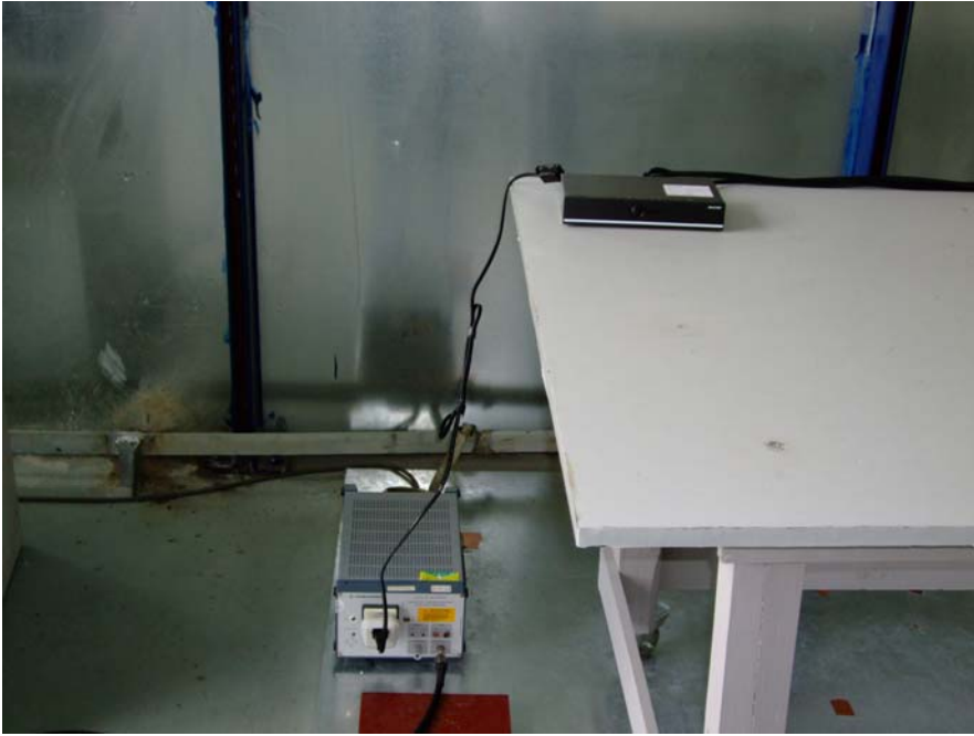
Conducted Emission Test Set-up Photo
