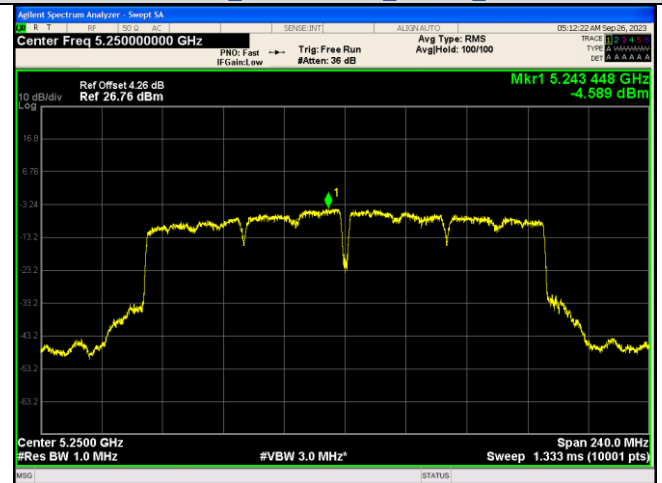
IEEE 802.11ac Channel 50 160MHz Antenna 0
