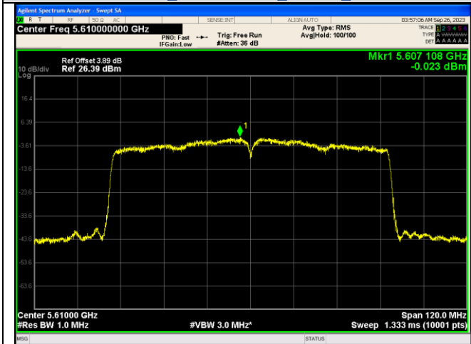
IEEE 802.11ac Channel 122 80MHz Antenna 2
