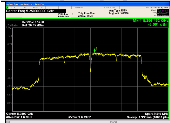
IEEE 802.11ac Channel 50 160MHz Antenna 2
