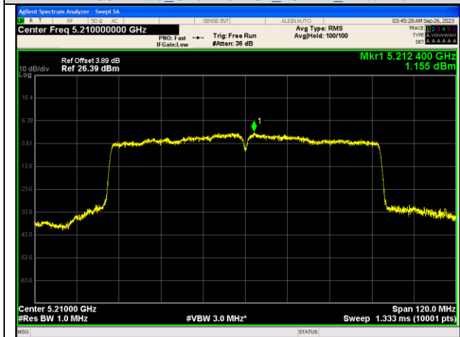
IEEE 802.11ac Channel 42 80MHz Antenna 2
