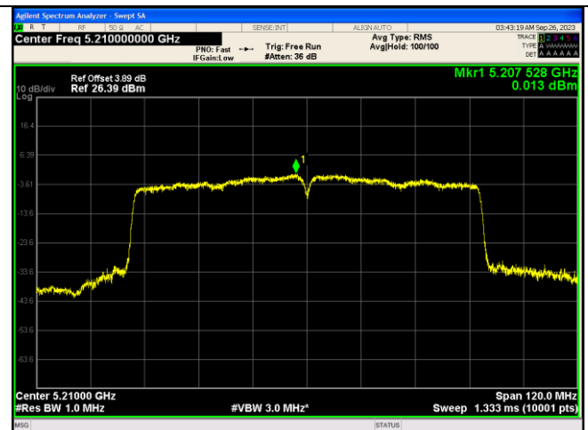
IEEE 802.11ac Channel 42 80MHz Antenna 0
