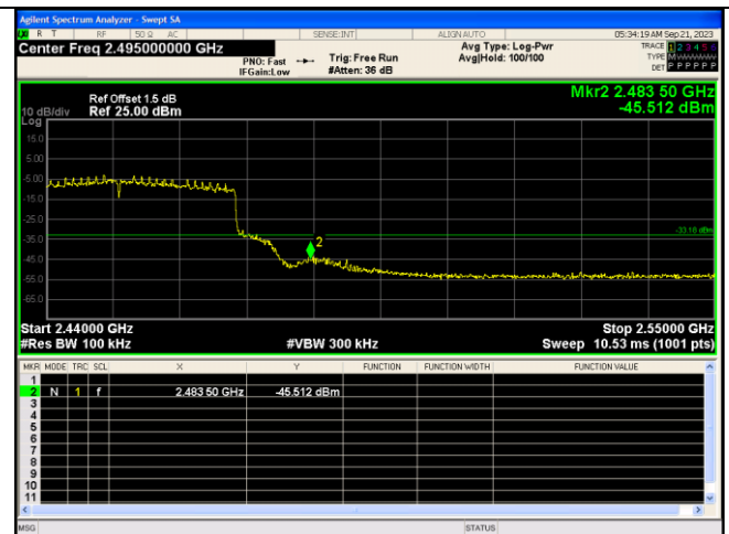
Out Of Band Emission IEEE 802.11ax_Channel 9_40MHz_Antenna 0_RU&Index 484RU65
