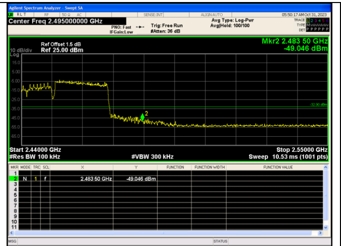
Out Of Band Emission IEEE 802.11ax_Channel 9_40MHz_Antenna 0_RU&Index 242RU62
