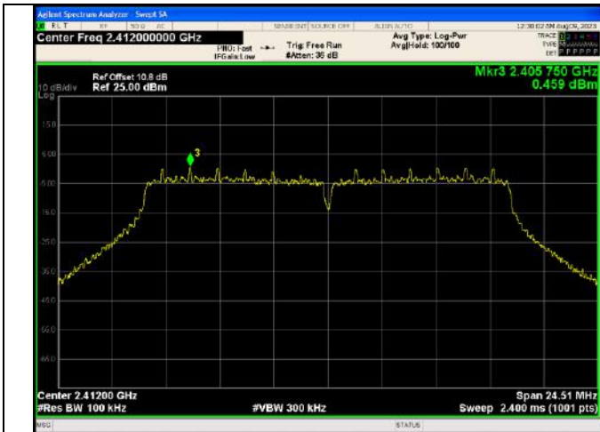
In-Band Reference Level IEEE 802.11g_Channel 1_20MHz_Antenna 0
