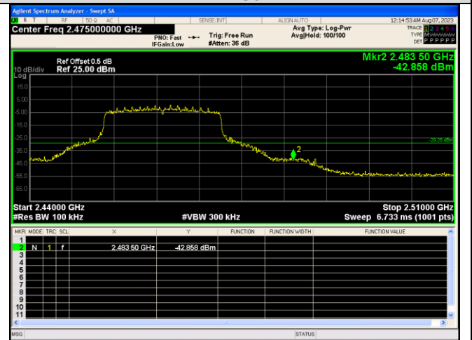
Out Of Band Emission IEEE 802.11ax_Channel 11_20MHz_Antenna 0_RU&Index 242RU61
