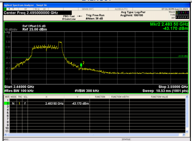
Out Of Band Emission IEEE 802.11ax_Channel 11_20MHz_Antenna 0_RU&Index 26RU8
