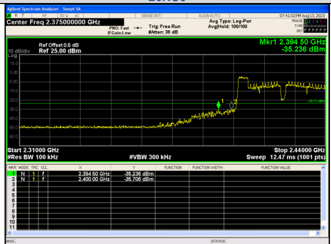
Out Of Band Emission IEEE 802.11ax_Channel 3_40MHz_Antenna 0_RU&Index 52RU37
