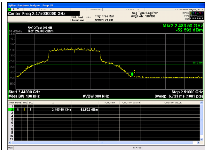
Out Of Band Emission IEEE 802.11ax_Channel 11_20MHz_Antenna 1_RU&Index 242RU61
