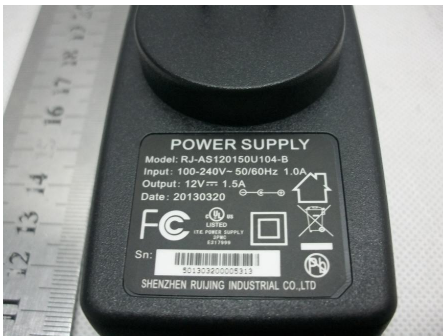
PHOTO OF POWER SUPPLY-1
