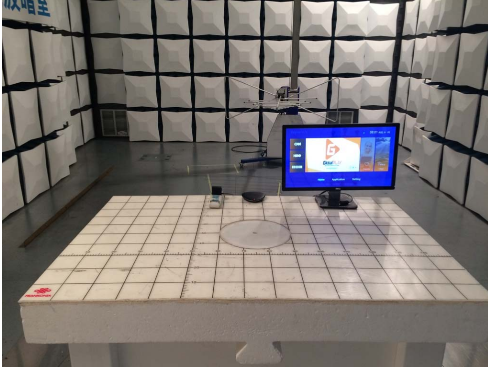
RADIATED RF MEASUREMENT SETUP (Above 1 GHz)
