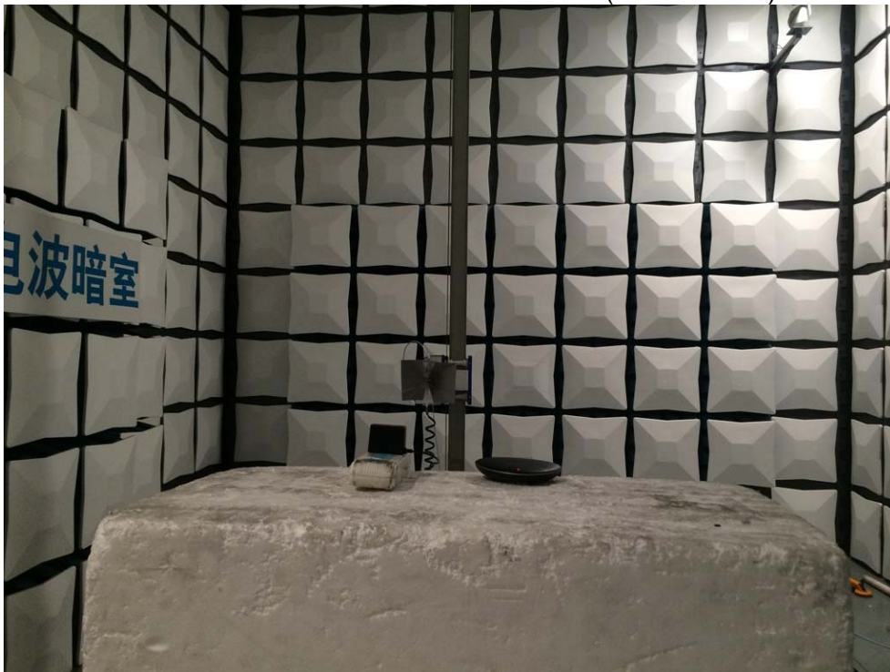
RADIATED RF MEASUREMENT SETUP (Above 1 GHz)
