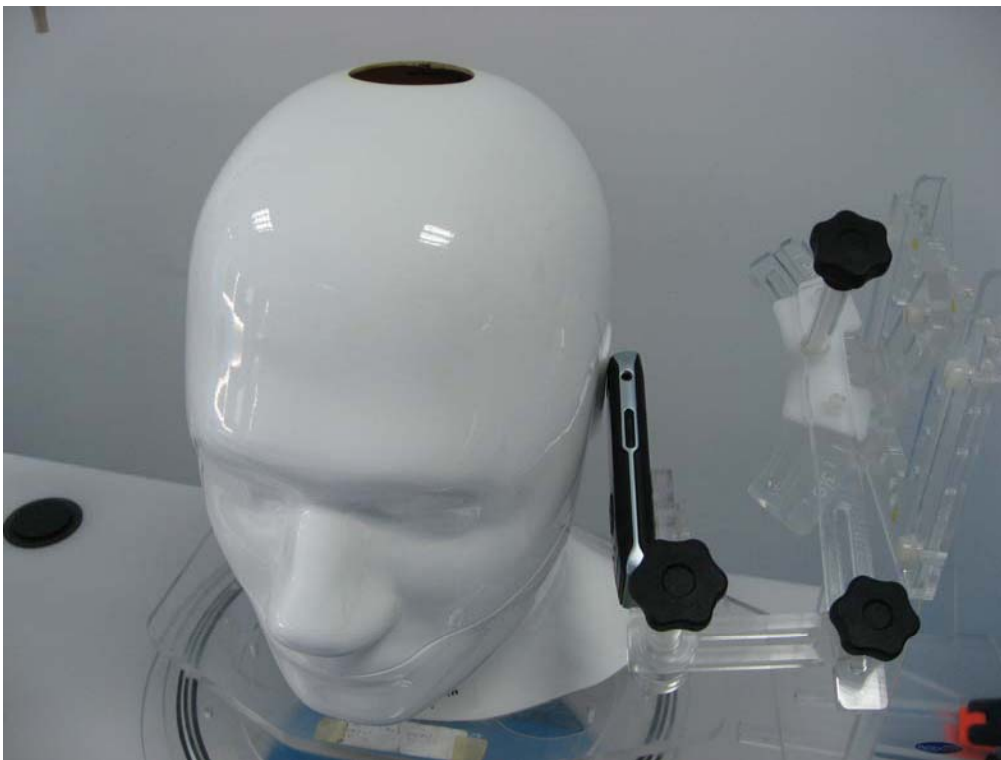
Fig.4 EUT Left Head Tilt15 Position
