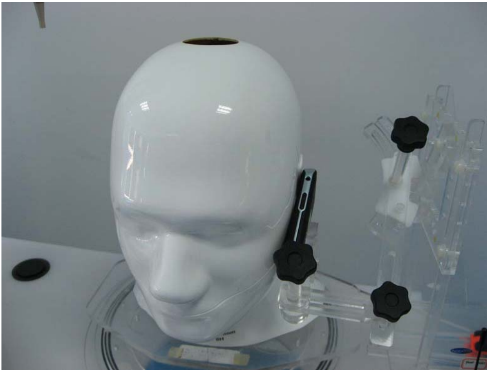
Fig.3 EUT Left Head Touch Cheek Position
