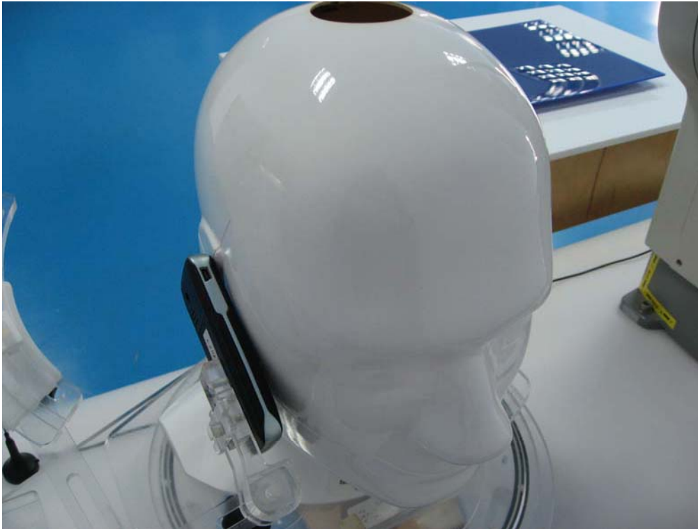
Fig.5 EUT Right Head Touch Cheek Position
