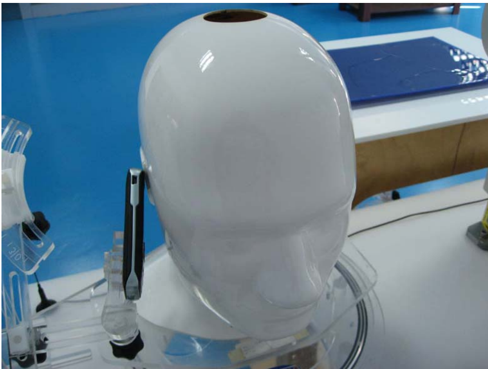
Fig.6 EUT Right Head Tilt15 Position
