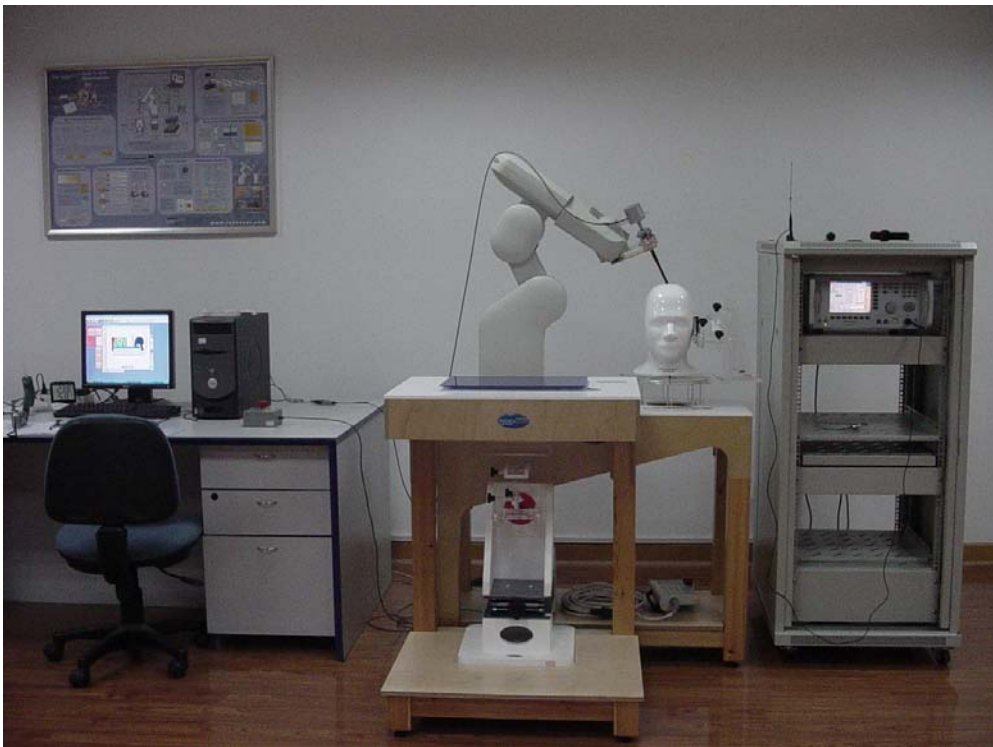
Fig.1 SARA2 System Test Layout
