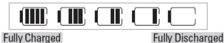
When the battery charge level becomes low, the low battery sensor will alert you in three ways: sounding an audible tone, blinking the battery icon outline, and displaying Low battery. Recharge soon, if the battery charge level becomes exceedingly low, the phone will automatically switch off and any function in progress will not be saved.
