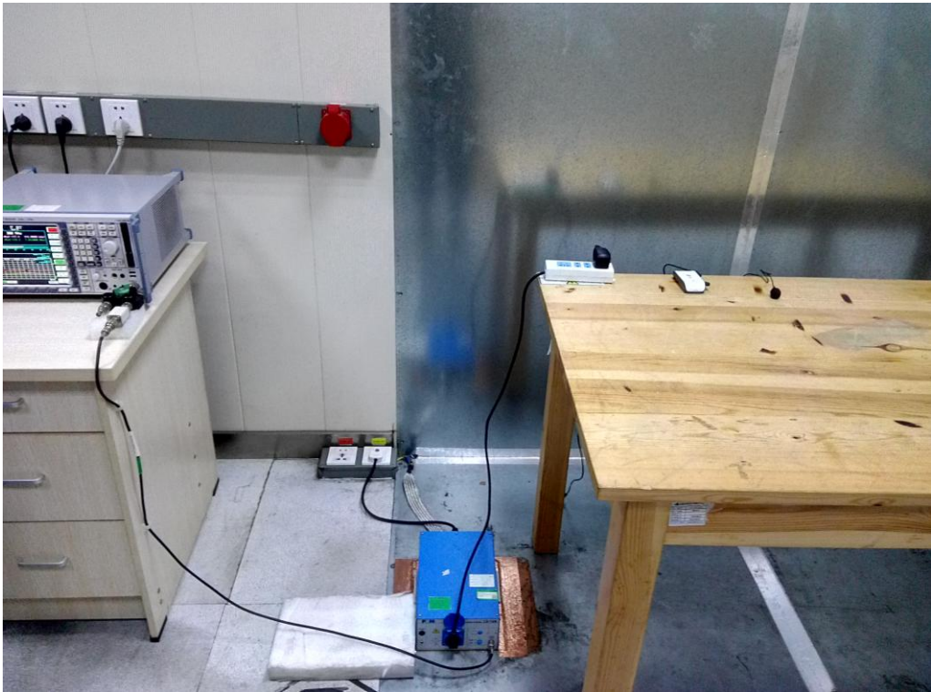
RADIATED EMISSION TEST SETUP BELOW 1GHZ
