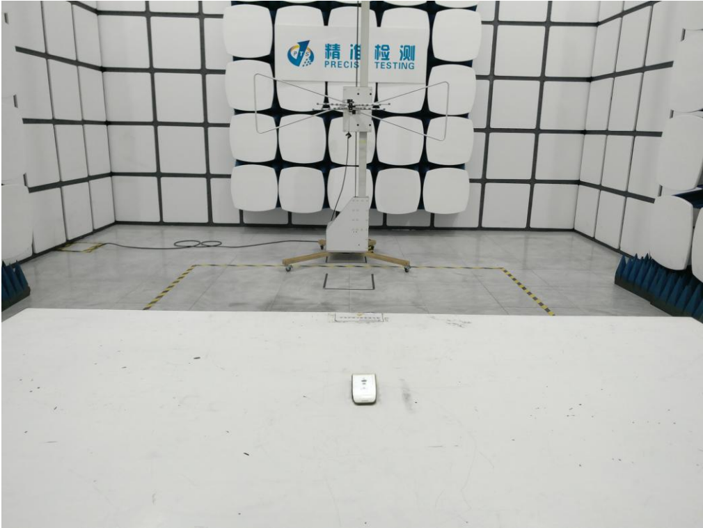
RADIATED EMISSION TEST SETUP BELOW 1GHZ
