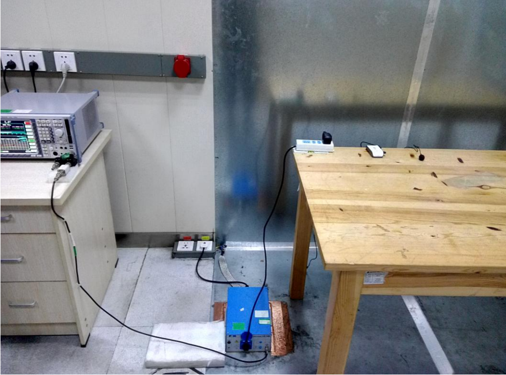
RADIATED EMISSION TEST SETUP BELOW 1GHZ
