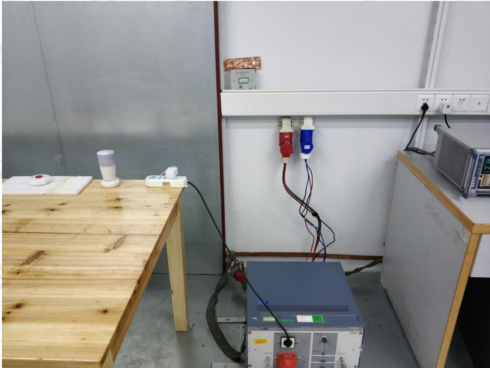
FCC RADIATED EMISSION TEST SETUP BELOW 1GHZ
