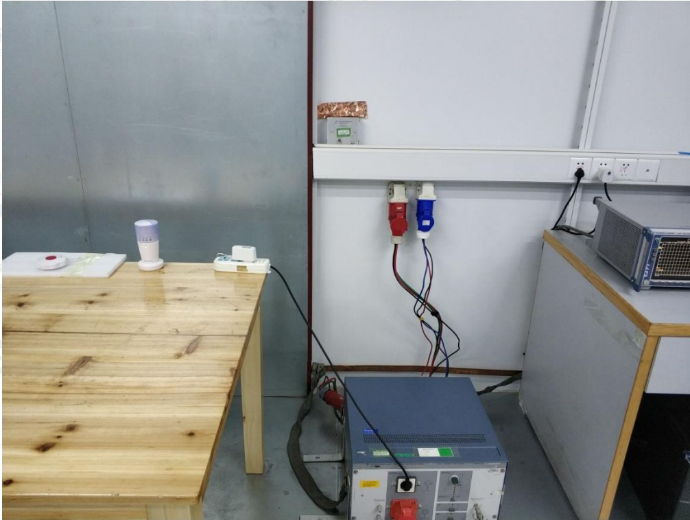
FCC RADIATED EMISSION TEST SETUP BELOW 1GHZ
