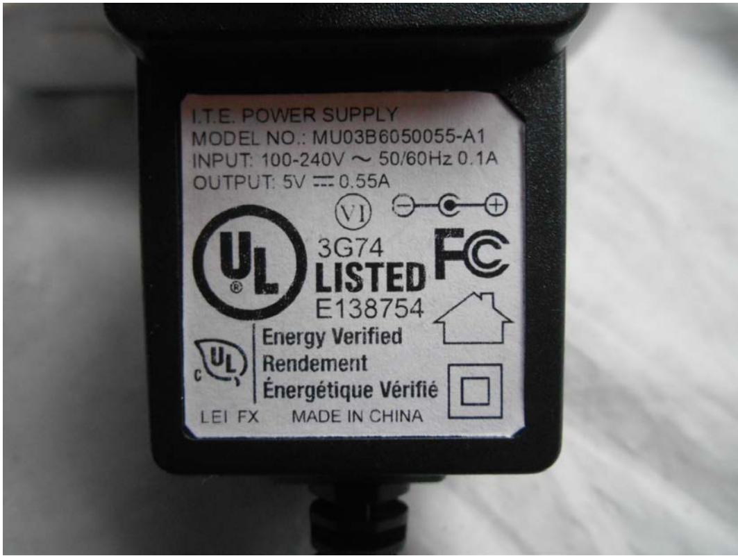
FIGURE 13 VISIT SMART HUB (M/N: BE1310) ADAPTER LABEL
