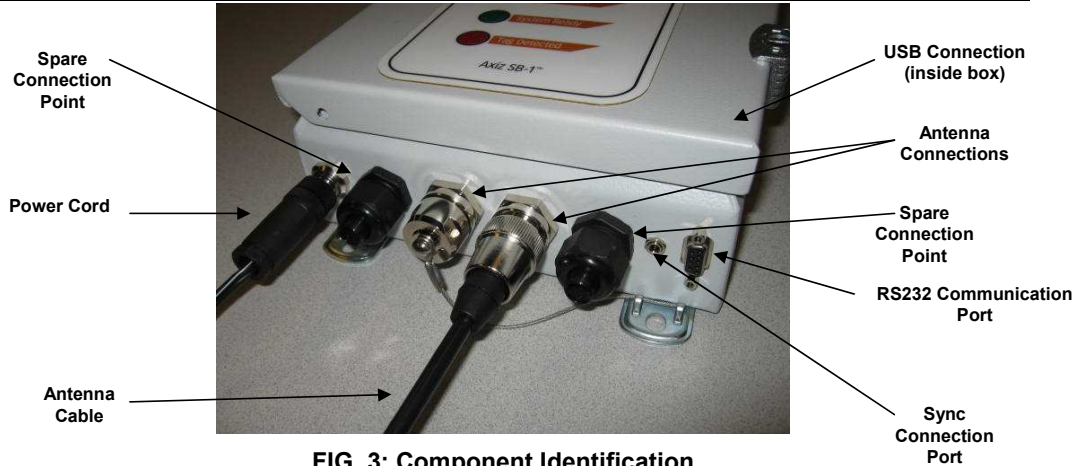
FIG. 3: Component Identification
