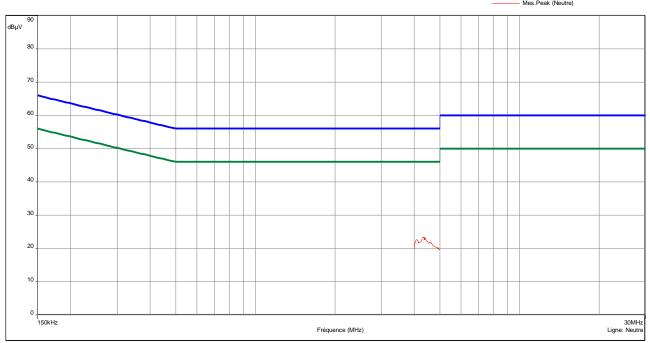
Curve N° 4: average measurement on the Line, for the frequency range: 4MHz to 5MHz
