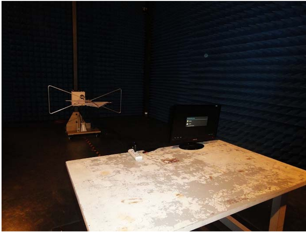
Radiated Emission Test Setup:
