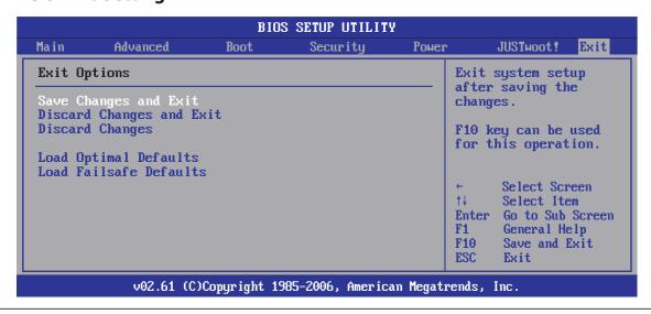
Highlight this item and select <Ok>,then press <Enter> to save the changes that you have made in the Setup Utility and exit the Setup Utility. Or press <Cancel> to return to the main menu.
