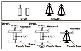
spacers. Take the tip of the spacers and insert them into the slots. After doing this to all the slots, you can slide the board into position aligned with slots. After the board has been positioned, check to make sure everything is OK before putting the chassis back on.
