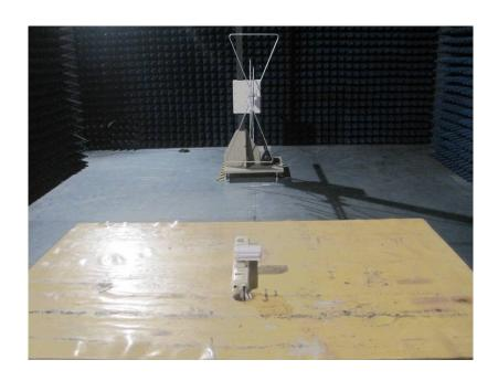
**Radiation Emission Test View For 1GHz-25GHz**
