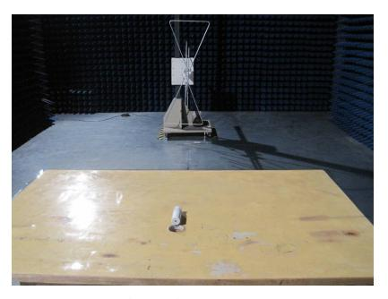
**Radiation Emission Test View For 1GHz-25GHz**
