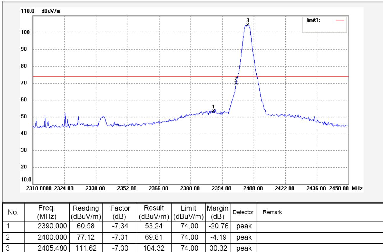
Remark: the mark3 is the fundamental in the test data.
