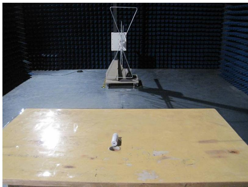
Radiation Emission Test View For 1GHz-25GHz
