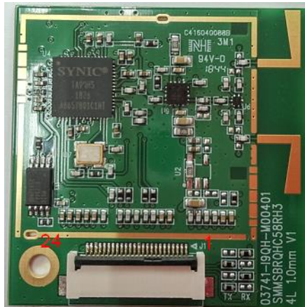
Fig 8.1 Pin sequence of SY5-A24-F Module
