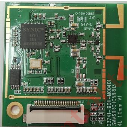
Fig 6.4 SY5-A24-F Module TX / RX without shielding case Top View
