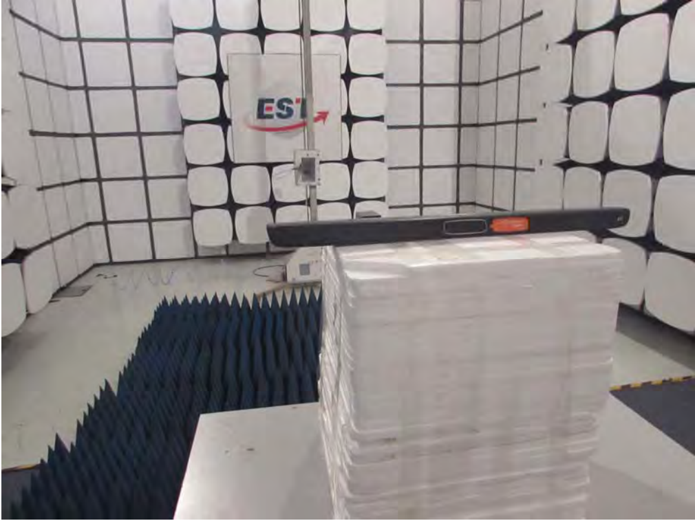
Radiated Test (1000-25000 MHz)
