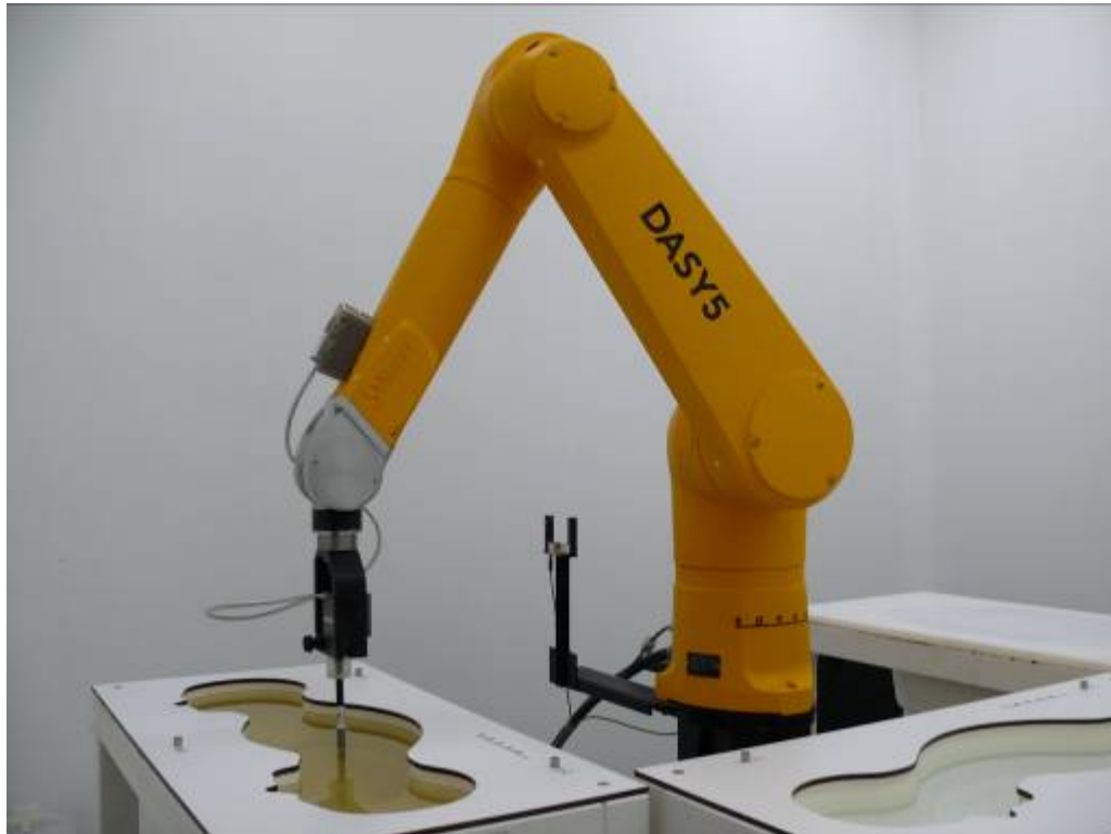
Picture 2: Specific Absorption Rate Test Layout
