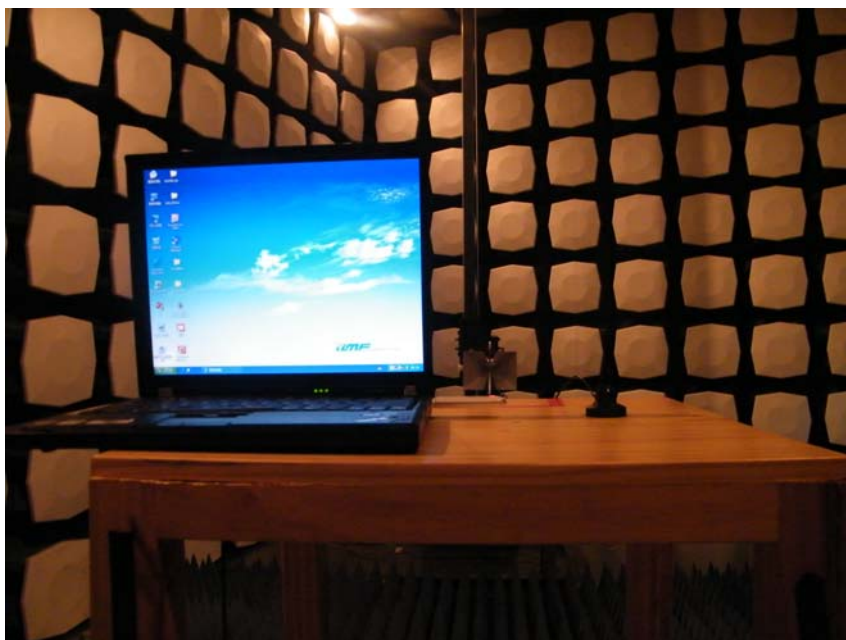
Picture 2: Radiated Spurious Emissions Test setup
